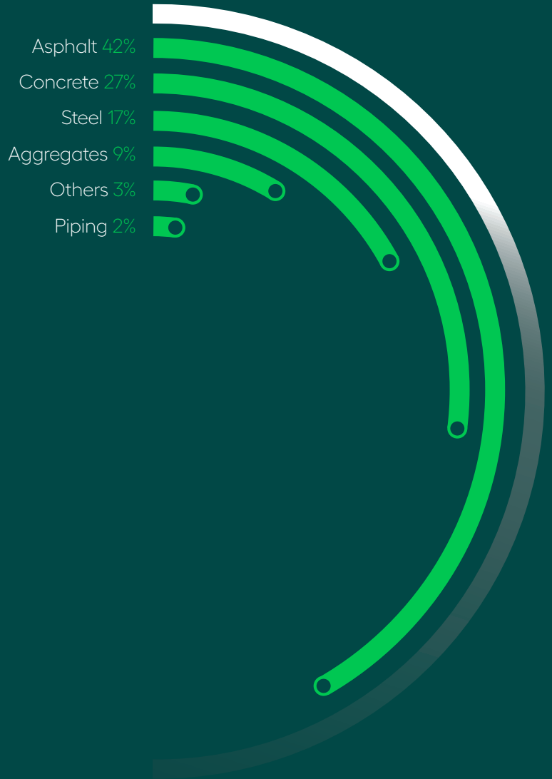
Figure 6: Embodied emissions contribution of materials for roads supply projects (Actual Case – As-Built data for roads)
