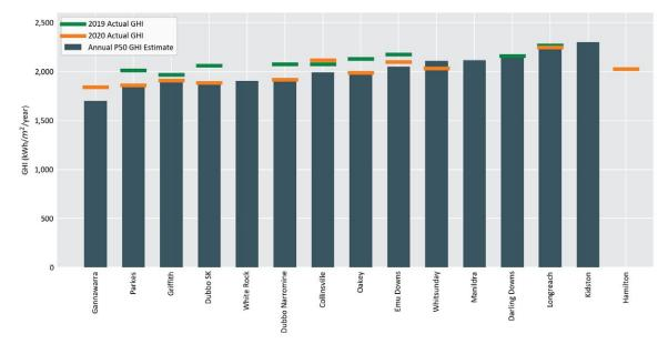
Figure 3. Forecast compared to actual GHI data for each of the LSS projects. NB not all Project's submitted complete data sets. Whitsunday forms an appropriate analogue for Hamilton in this plot due to their similar size and geographic location.
