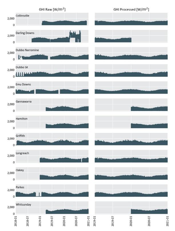
Figure 2. Raw measurements provided for global horizontal irradiance by each LSS proponent before and after data processing to get one, or two where possible, years of clean irradiance data.
