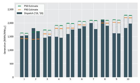
Figure 1. Comparison of AEMO's records for actual energy dispatched (TOTALCLEARED) and estimates for generation across the LSS portfolio for year 2019 and 2020. NB Project 7 did not submit a P90 estimate.
