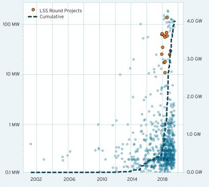
Figure 3. Solar PV systems greater than 100 kW accredited by the CER in Australia. Ekistica analysis of data from the Australian Photovoltaic Institute<sup>3</sup>
