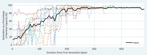
Figure 6. LSS Round Projects ramping up generation over time, where each line represents a different project. Note that each data point represents the power system's maximum dispatched power each week and has not been seasonally adjusted.
